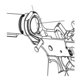
• DEPRESS THE BUFFER RETAINER PIN TO PERMIT THE BUFFER AND THE SPRING TO MOVE FORWARD. DEPRESS THE HAMMER TO ALLOW THE SPRING AND THE BUFFER ASSEMBLY TO CONTINUE MOVING FORWARD AND BE REMOVED FROM THE RECEIVER EXTENSION.
