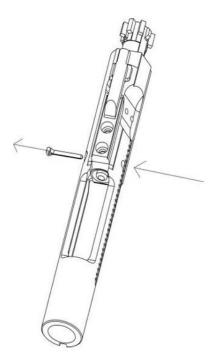
• TILT THE BOLT FACE UP AND REMOVE THE FIRING PIN.
