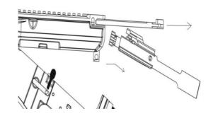
• REMOVE THE CHARGING HANDLE BY PULLING IT BACKWARDS TO KEYWAY AND THEN DOWN AND OUT OF THE UPPER RECEIVER.
